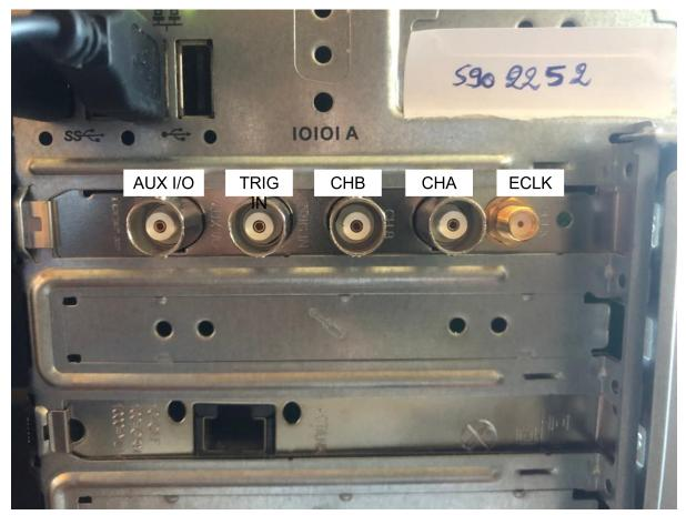
The AUX I/O port can be configured using aux\_io\_mode and aux\_io\_param.
